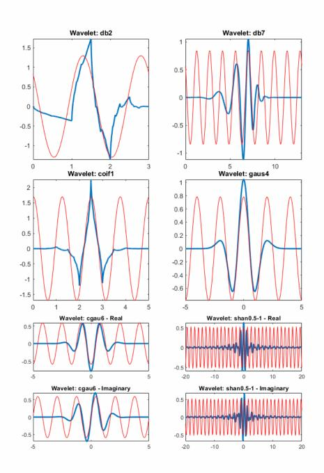
As you can see, the center frequency-based approximation (red) captures the main wavelet oscillations (blue). The center frequency is a convenient and simple characterization of the dominant frequency of the wavelet.
